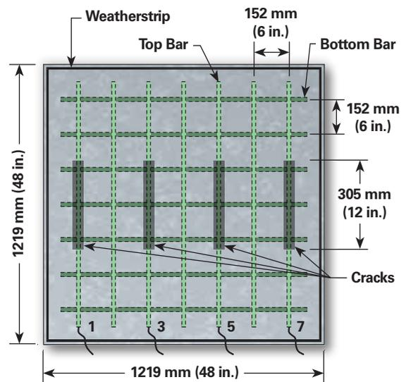
Field Test Specimen Setup —
