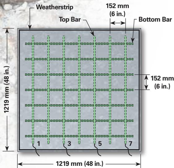
Field Test Specimen Setup —
