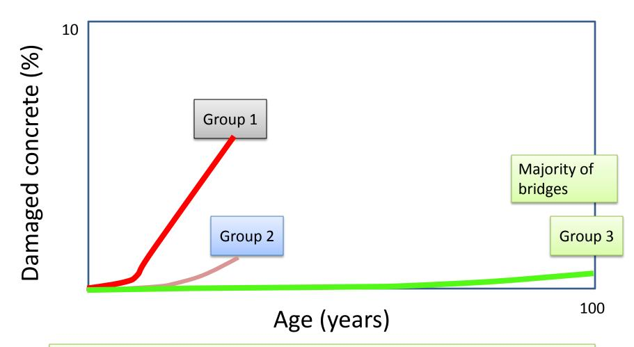
Most structures containing epoxy reinforcement are **predicted to have a 100 year life**
