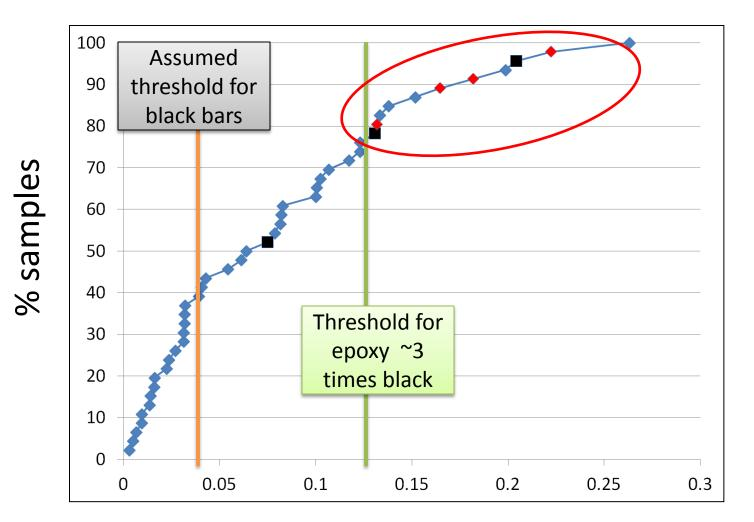
Chloride (% by weight concrete)
