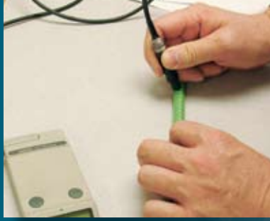
Epoxy-coating thickness test.
