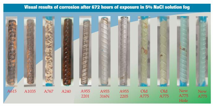
All bars tested 'as received' except the epoxy-coated bar indicated had a 1/16 inch hole drilled
