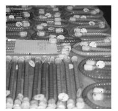
as solution testing to study coating adhesion. The ten that performed the best were picked for further evaluation.
