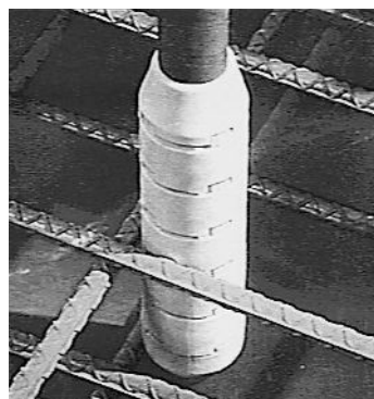
Non-metallic vibrator head
