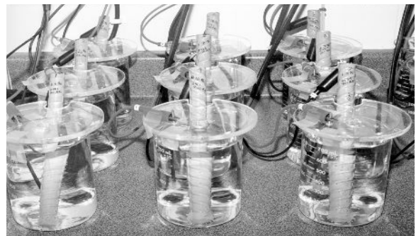
Cathodic Disbondment testing
