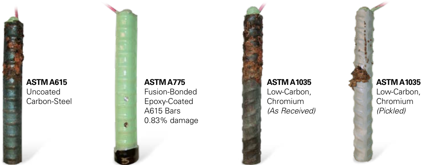
Figure 5: Visual condition of bars at the end of the testing program. Note the minimal corrosion of the epoxy-coated bars compared with those of the ASTM A615 and A1035 bars.
