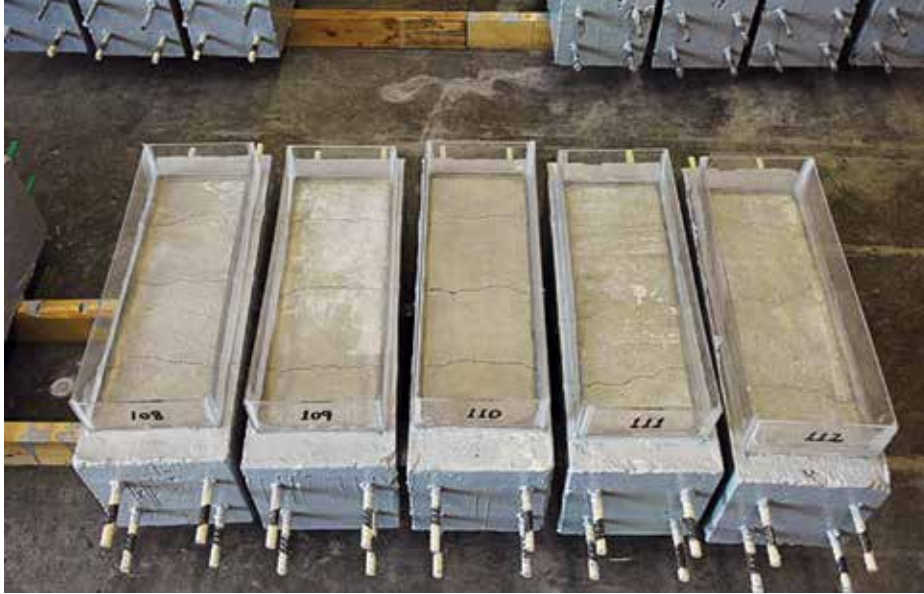
Cracked Concrete Macrocell Under Preparation For Corrosion Testing.
