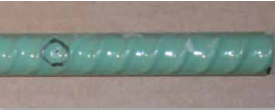
Figure 6 Epoxy-coated reinforcing steel (mashed) in OPC after impressed current test.
