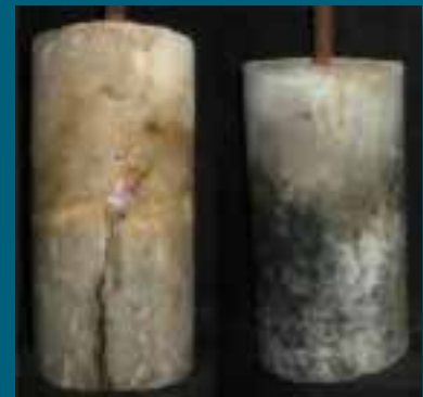
Figure 1 Visual comparison of ternary vs OPC specimens containing carbon-steel bars.
