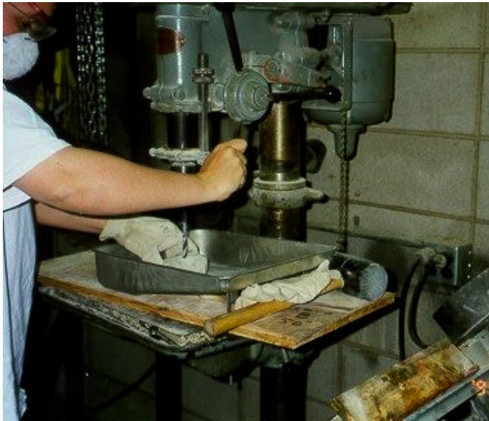
Figure 4.8 Collection of Powder Samples
