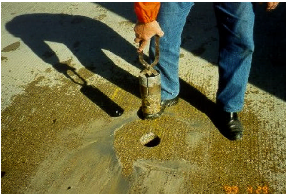
FIGURE 4.4 Extracting the Core
