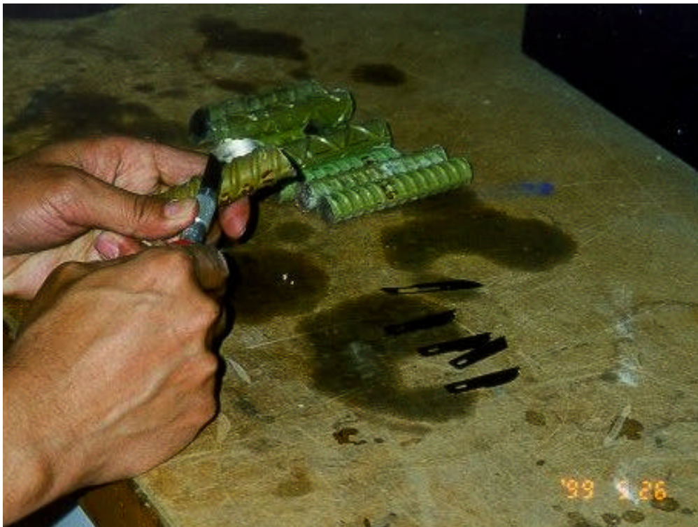
FIGURE 4.10 Epoxy Coating Bond Test
