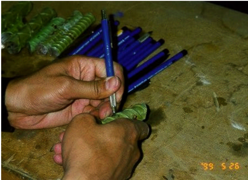
FIGURE 4.9 Coating Hardness Test
