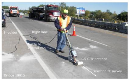
Researchers used ground penetrating radar (pictured), impedance spectroscopy and half-cell potential measurements in the field to evaluate the level of corrosion of the bars.
