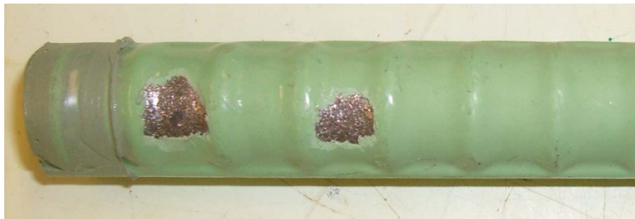
Figure A3: 0.04% ECR, specimen 2, side B. After disbondment. Disbonded areas close to the average ( 42 \text{ mm}^2 ) for 0.04% ECR specimens (see Table A1a).
