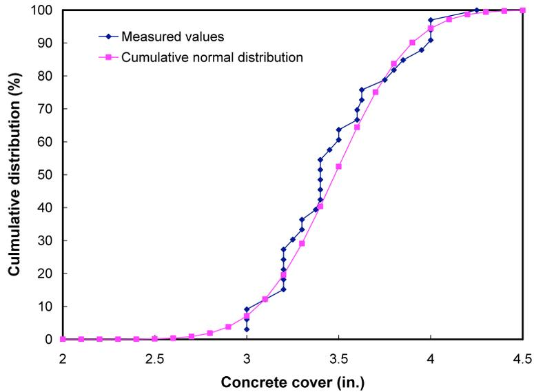
Figure 9. Measured values and fitted cumulative cover thickness normal distribution of the MacKay River Bridge substructure.
