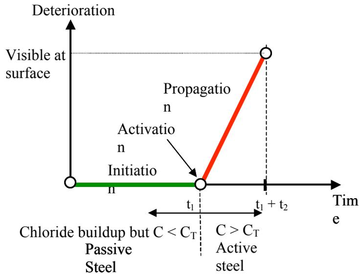
Figure 2. Corrosion sequence (Tuutti 1982)
