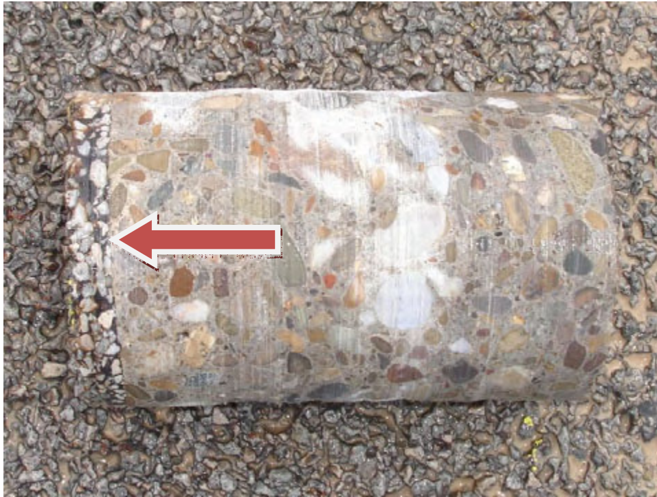
Figure 9. Thin polymer overlay visible on top (left) of core from Bridge No. 2668N.
